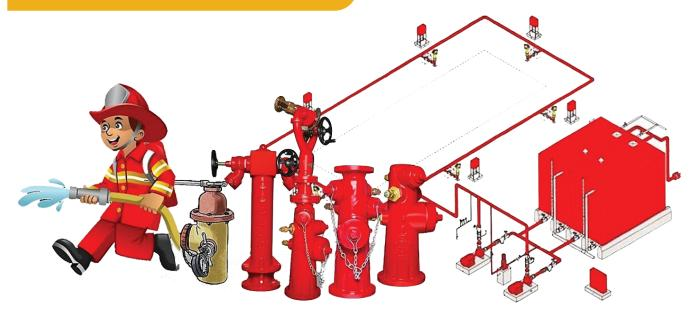
Standpipe systems are a network of piping in a building fed by a water supply and featuring numerous outlets for the water. They are essentially indoor fire hydrants that allow occupants, firefighters, or both to access water to fight fires.
